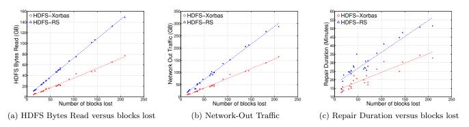
Figure 6: Measurement points of failure events versus the total number of blocks lost in the corresponding events. Measurements are from all three experiments.
